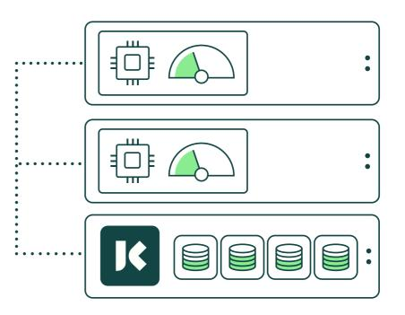
Disaggregated scale-out NVMe storage appliances enable multiple NVMe devices to function as a logical storage pool with logical volumes allocated to any application across the network. Designed to be dynamically reconfigurable, disaggregated storage architectures enable physical resources to be reconfigured to maximize performance and minimize latency.
